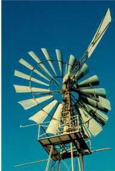
*American windmill used for water pumping, © Bundesverband WindEnergie e.V.*
